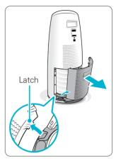
② Once the back panel is removed, grasp the handle near the bottom of the unit, and pull towards yourself to lower and release the filter.
